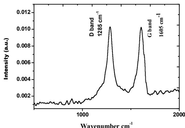
**Fig .4 Raman spectrum of h-MWCNTs**
