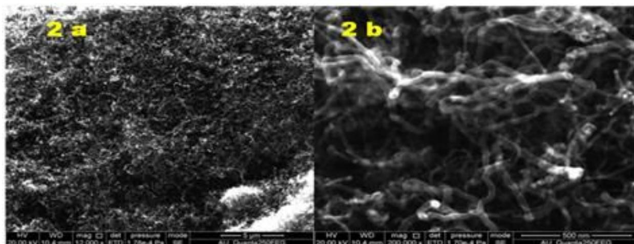
**Fig. 2 SEM images of CNTs a) bundle of CNTs b) CNTs with helical shape**
