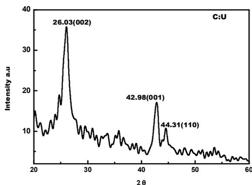
**Fig. 1. XRD of synthesized CNTs using C:U combustion fuel**
