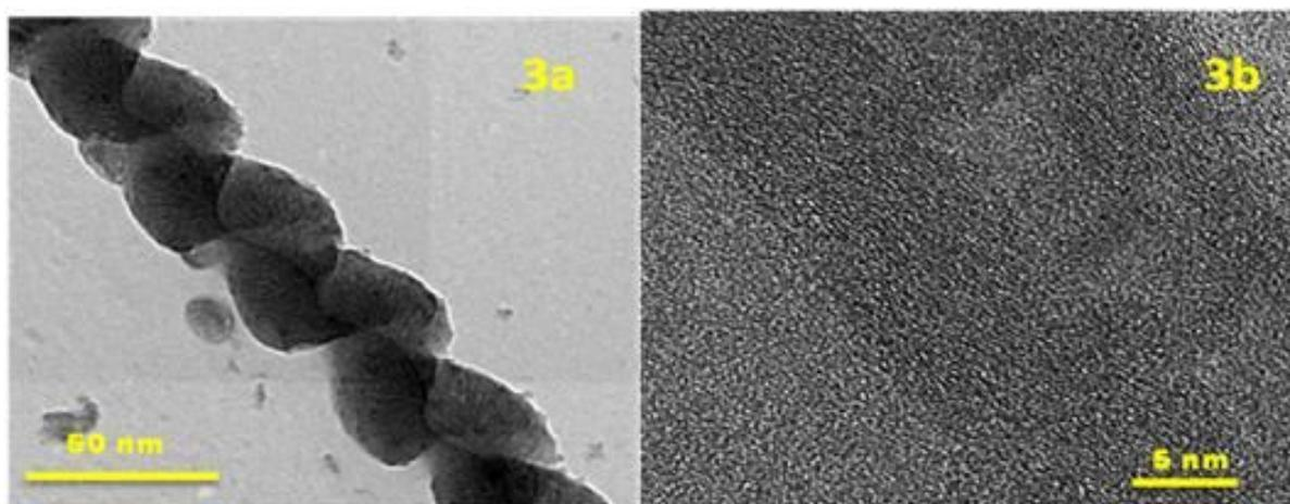
**Fig. 3 HRTEM images of CNTs a) helical CNTs b)high magnification of h-MWCNTS**
